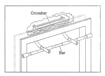
▲ WARNING: The door gym is designed to fit door frames with a width of 27.5–30 inches (70–78 cm) and a depth of 4.5–6 inches (11–16 cm). Do not install the door gym in a door frame that does not meet these specifications. The crossbar must rest on the top edge of the door frame when the door gym is installed in the high position.
